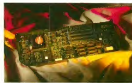
The G-Force card is much more than just an accelerator - it has a SCSI interface too.
